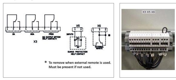
When an alarm occurs, the X3 relay contacts are de-energized and switch.
