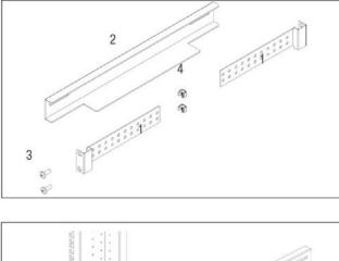
4x Fixing brackets (ref 1) 2x Slider (ref 2) 12x Mounting screws (ref 3) 12x Cage nuts (ref 4)
