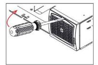
A) Use screwdriver to release the latch
